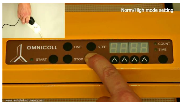
Figure 3.7-1 Press the SET button on the control unit and connect the plug-in power supply to the mains.
