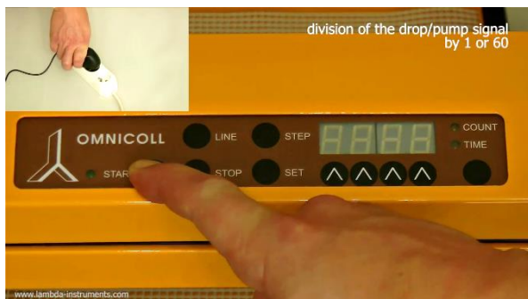
Figure 3.4-10 Press the button START while plugging the power supply into the mains.
