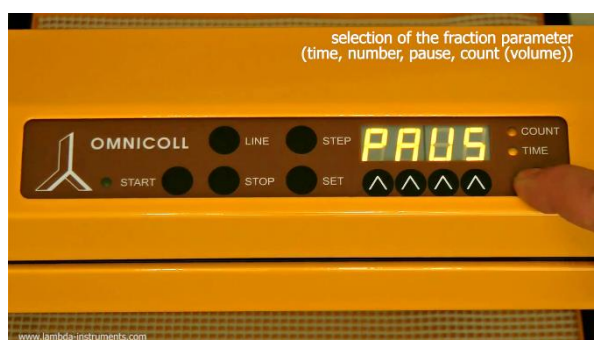
Figure 3.7-6 Selecting the parameter PAUSE for introducing pauses in the program. [Count LED: ON; Time LED: ON; Display: PAUS]
