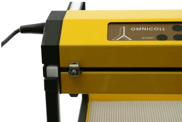
Figure 3.8-4 Unscrew the tubing guide holder screw on the moving arm of the OMNICOLL fraction collector
