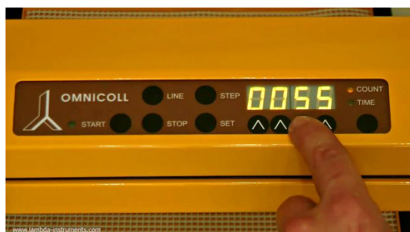
Figure 3.6-3 Select the desired count number with the button \wedge \wedge \wedge \wedge under the display, for example: 55.
