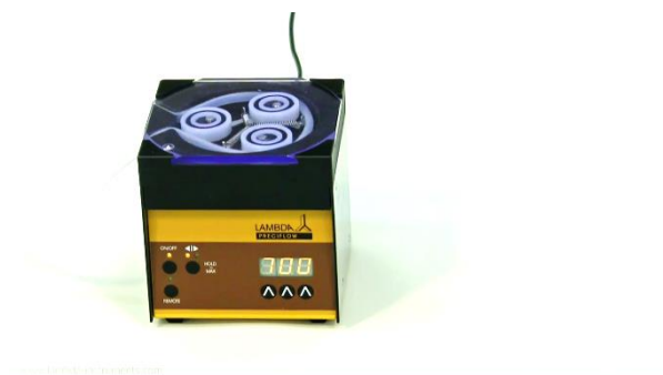
Figure 3.6-5 Select the speed control on the peristaltic pump (e.g. 700), choose the pump rotation direction and switch the pump on.
