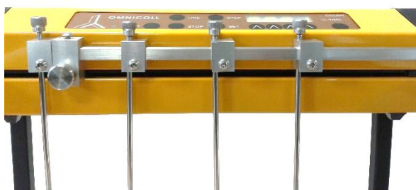
Figure 3.8-10 Place the tubing guide holder at the desired fraction position and secure it with the socket head screw using the corresponding socket key (Allen key).
