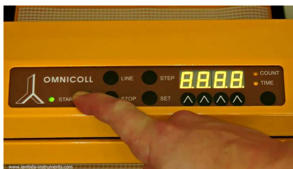
Figure 3.6-6 Press the START button on the collector to start fraction collection. If the tubing was not filled completely with the liquid, for example water, take a second fraction.
