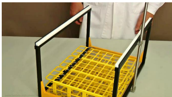
Figure 3.3-5 Mark the row distance with a pencil on the coding band for Y-axis and draw the white lines with the provided correction pen.
