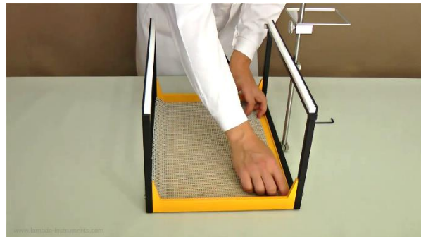
Figure 1.1-8 Place the fixing mat in the support. When needed clean the mat from dust and dirt with a humid cloth. Make sure that the mat is dry before use.
