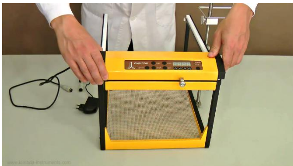
Figure 1.1-9 Place the control unit just at the beginning of the gear rails. The distance from the edge should be the same on the left and right sides. The gear wheels of the control unit must engage correctly in the gears of both rails. Be sure that nothing will disturb the movement of the control unit during fractionation.
