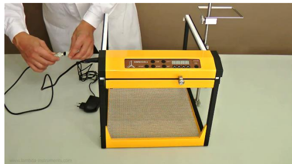
Figure 1.1-10 Connect the cable of the control unit of the LAMBDA OMNICOLL fraction collector and sampler with the cable of the power supply plug.
