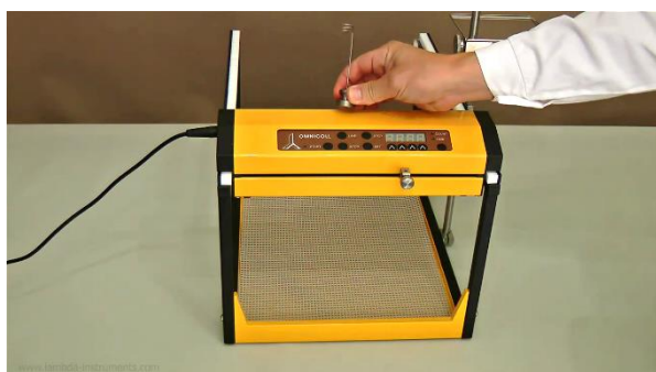
Figure 1.2-1 Place the magnetic tubing holder conveniently in the center of the fraction collector carriage and control unit.
