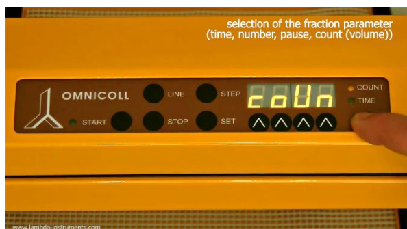
Figure 3.7-4 Selecting parameter COUNT (volume). [Count LED: ON; Time LED: OFF; Display: coUn]
