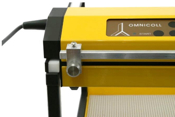
Figure 3.8-6 Insert the rectangular bar into the bar holder as shown.
