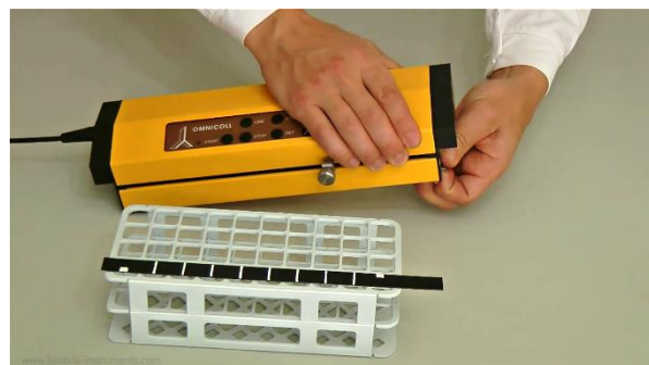
Figure 3.3-4 Place the coding band in the X-axis holder and insert into the desired slot of the control unit, with white stripes facing up.
