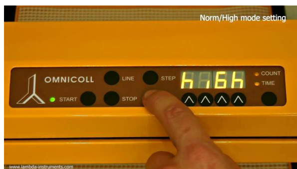
Figure 3.7-3 Confirm the selection by pressing the SET button (long beep signal).
