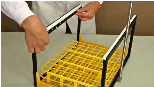
Figure 3.2-1 Place the longer and narrower coding band (Y-axis) on the left inner metal frame just under the gear-bar as shown. The first coding line should lie approximately 10cm from the front frame.
