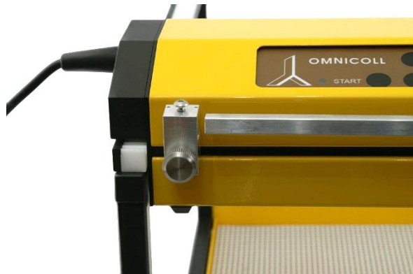
Figure 3.8-5 Place the bar holder on the tubing guide holder screw.
