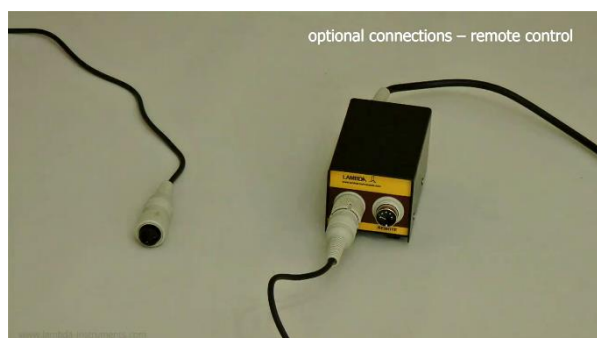
Figure 3.6-1 Connect the peristaltic pump remote control cable to the communication module box.
