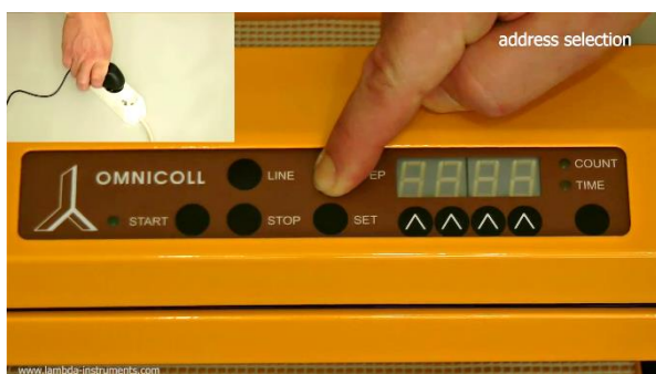
Figure 3.4-14 While keeping the direction button STEP pressed connect the fraction collector to the mains.
