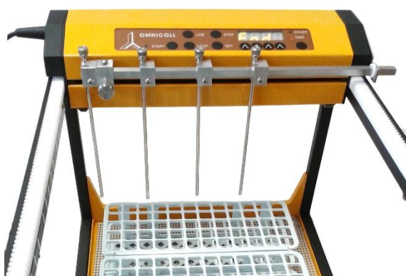
Figure 3.8-11 Place the tubing guide holder in position above the first fraction of each stream (channel).
