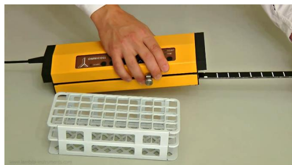
Figure 3.2-4 Insert the X-axis holder with coding band into the desired slot of the control unit, with the white coding stripes facing up.
