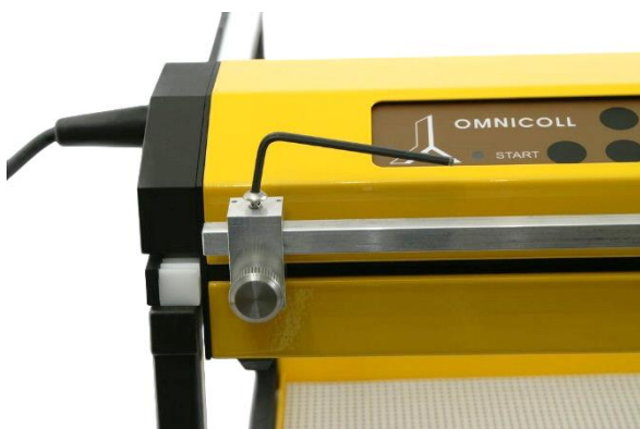
Figure 3.8-8 Screw the bar holder on the moving arm of the fraction collector with the corresponding socket key (hex-key). Use e.g. a thin spatula to push the screw through the moving arm.
