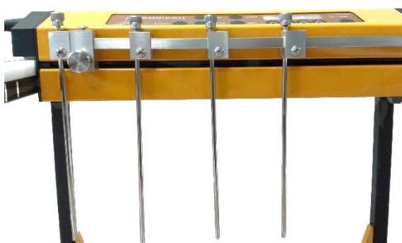
Figure 3.8-9 Slide the tubing guide into the tubing guide holder, so that a convenient height above the tubes is obtained.
