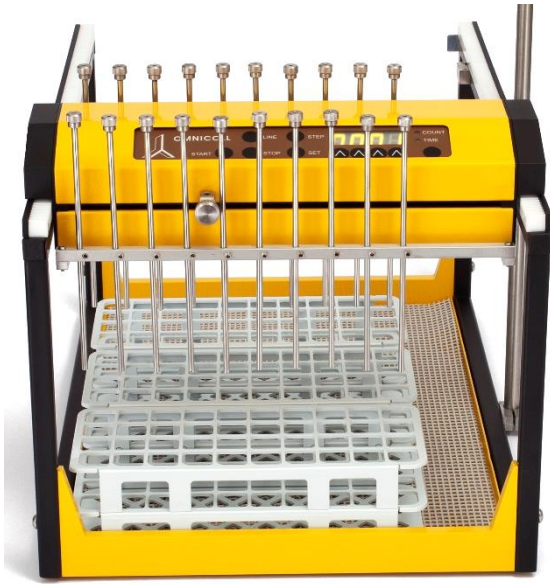
Figure 3.8-3 Example of taking 20 simultaneous fractions in a 20-stream (channel) configuration
