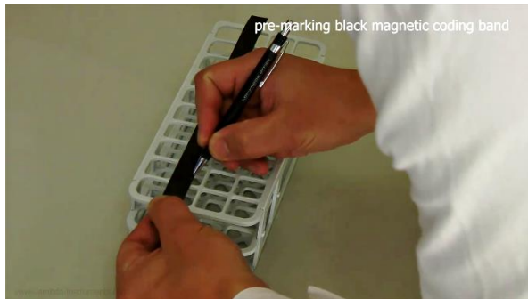
Figure 3.3-1 Place the coding bands on the tube rack and mark the fractioning position with a normal pencil.
