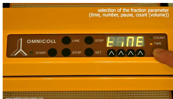
Figure 3.7-5 Selecting the parameter TIME to perform the program for a desired time. [Count LED: OFF; Time LED: ON; Display: tiMe]
