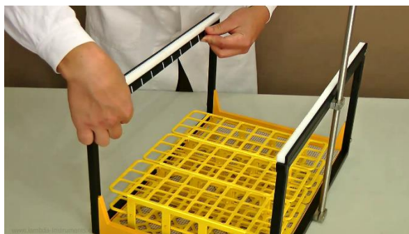
Figure 3.3-6 Place the coding band on the left internal side of the metal frame just under the gear bar.
