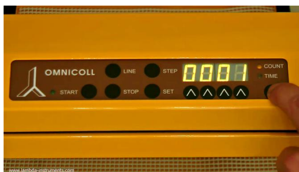
Figure 3.6-2 With the COUNT/TIME button select the count modus (the COUNT LED will be switched ON)
