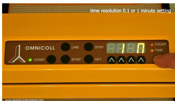
Figure 3.4-7 The actual time resolution will appear on the display " 0.1M " or " 1M ".
