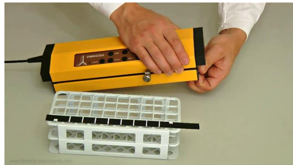
Figure 3.2-2 Pull the X-axis coding band holder from the OMNICOLL control unit as shown.
