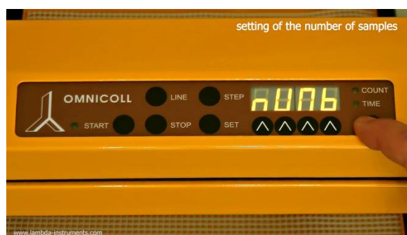
Figure 3.7-7 Selecting the parameter NUMBER for collecting a number of samples. [Count LED: OFF; Time LED: OFF; Display: nUMb]
