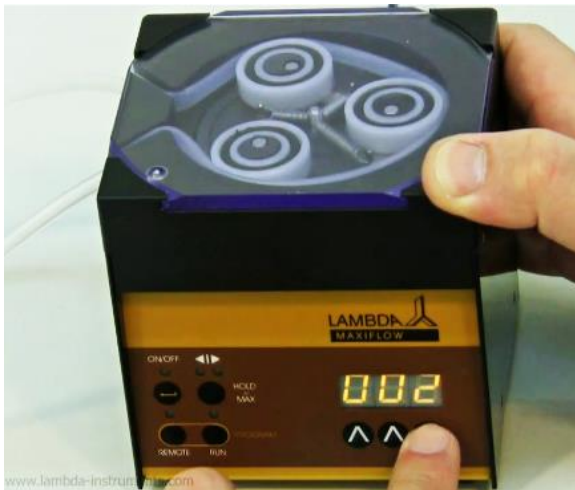
Figure 2-7 Select the desired time period for the first program step by pressing the buttons \blacktriangle below the display (from 0 to 999 minutes or 00.0 to 99.9 minutes).
