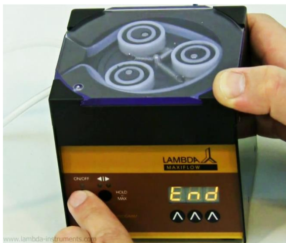
Figure 2-19 Press the ON/OFF button until the indication “End” appears on the display to confirm and save the program.
