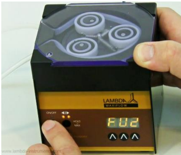
Figure 2-9 Press the ON/OFF button. The indication “F02” will briefly appear on the display.
