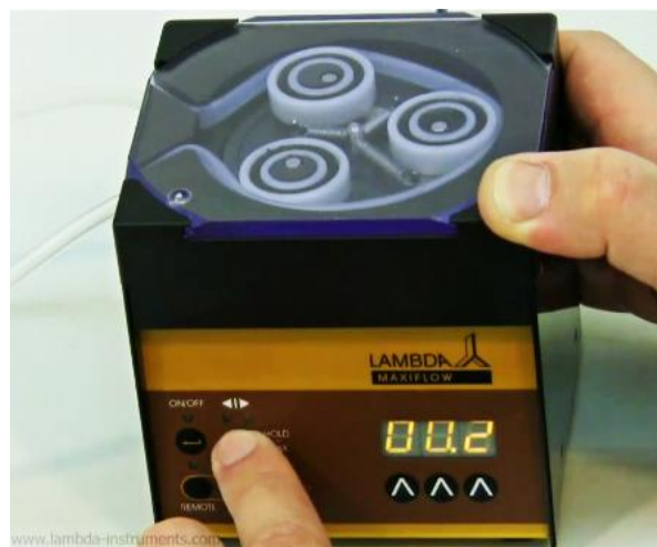
Figure 2-14 Press ◀▶ button, to set the time resolution.
