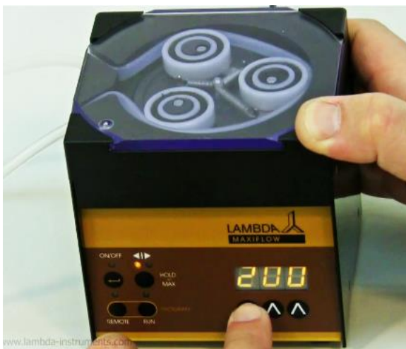
Figure 2-11 Enter the desired flow rate for the second program step.
