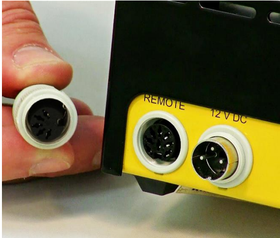
Figure 1-1 Plug the connector of the power supply into the corresponding socket (12 V DC) at the rear of the peristaltic pump and secure it.
