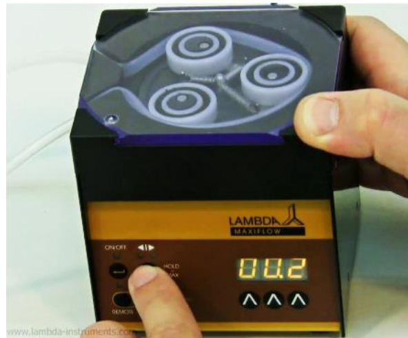
Figure 2-8 By pressing the \blacktriangleleft button, the time resolution can be set in minutes or 0.1 minutes. In the 0.1 minute time resolution a dot is displayed, e.g. “00.1”. The time resolution can be set individually for each program step.
