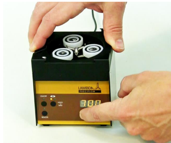
Figure 1-4 The speed of rotation has to be increased using the “^ ^ ^” arrows present below the LED display. Set the pump speed to about 700. The speed range of about 300-700 for tubing insertion can be used.
