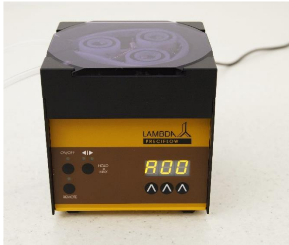
Figure 4-4 The message “A” and two numbers will appear on the display. This number from 00 to 99 is the current address of the pump.
