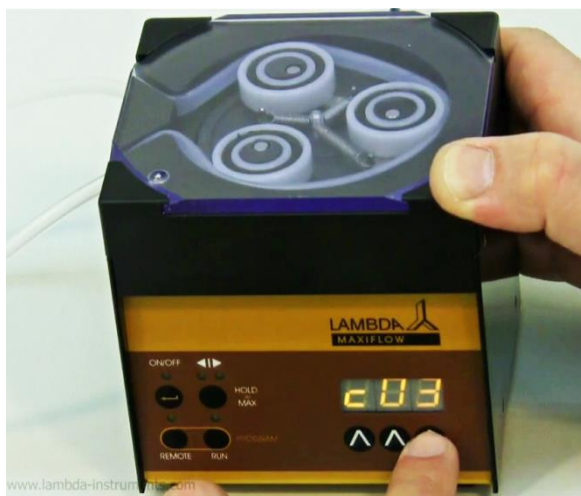
Figure 2-18 If you wish to repeat the same program 3 times, increase the cycle number to “c03” by pressing the buttons ^ ^ ^ below the display (from 0 to 99 cycles). The program can be repeated up to 99 times, indicated by “c99” . If 0 is entered for the cycle number “c00” , the program will run continuously (infinite loop).
