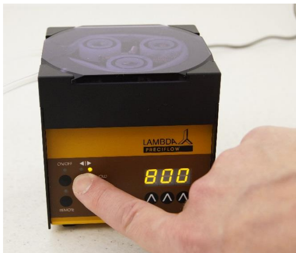
Figure 1-14 LED illumination in the direction |▶ represents the anticlockwise rotation.
