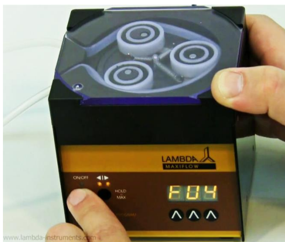
Figure 2-15 After having entered the time of the last step, press the ON/OFF button.
