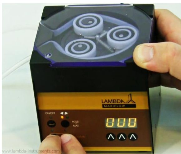
Figure 2-16 The flow rate ( 000 ) of the next step which will not be programmed appears on the display.
