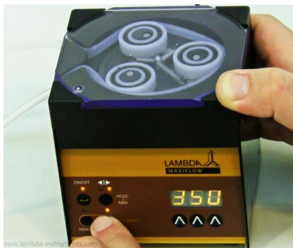
Figure 2-20 To start the program, press the RUN button. The RUN and ON/OFF LEDs are on. To stop the running program definitively, press the RUN button. The RUN and ON/OFF LEDs are off
