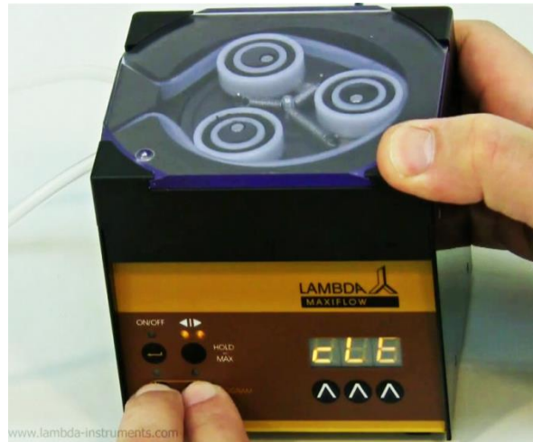
Figure 2-2 Continuous pressing of REMOTE and RUN button even after the indication of “ PGM ” ends up with the “ cLE ” indication.
