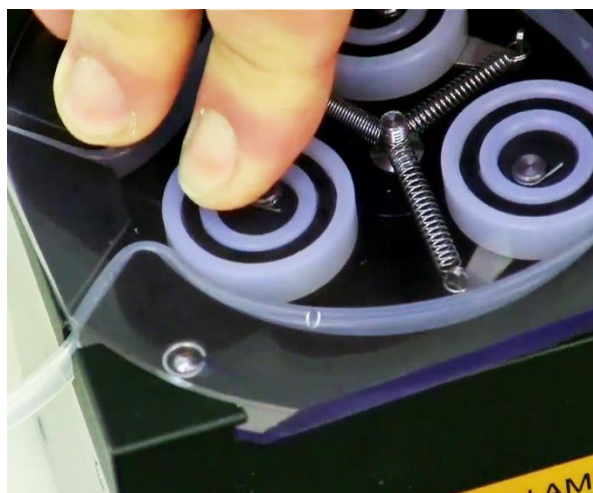
Figure 1-10 Turn the cover so that the steel ball embedded in the left-front corner of the peristaltic pump fits into the notch in the cover.
