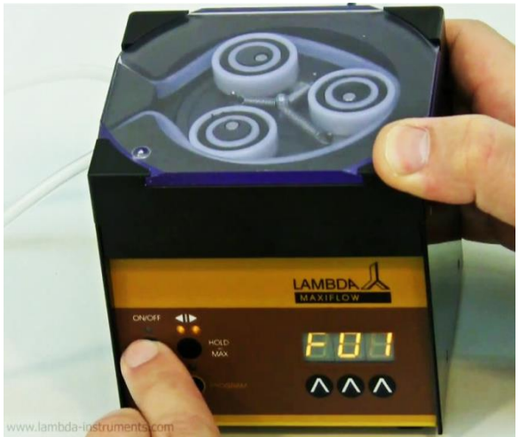
Figure 2-3 Press the ON/OFF button. The indication “ F01 ” will appear for a short time on the display indicating that you can select the first flow rate (speed setting) value.
