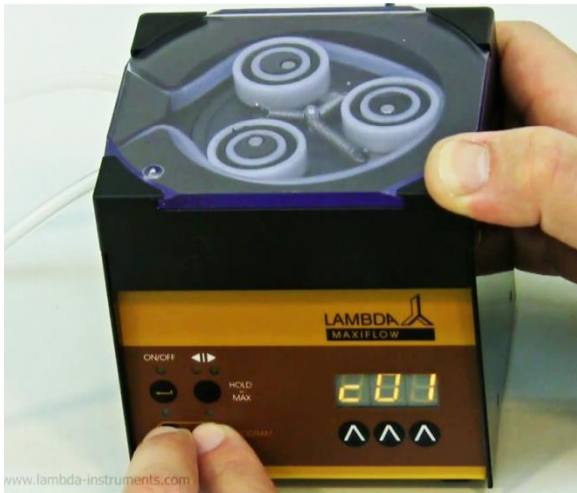
Figure 2-17 Press the Remote and Run button simultaneously and you will see the indication " c01 " on the display. This indicates that the program will be executed only once and the peristaltic pump will stop afterwards.
