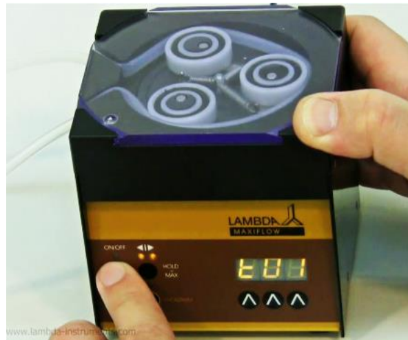
Figure 2-6 Press the ON/OFF button. The indication “t01” will appear for a few seconds on the display indicating that you can program the time period of the first step in minutes.
