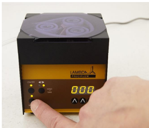
Figure 4-2 Press the button REMOTE on the front panel. The corresponding LED diode will go on and the display will indicate the approximate voltage of the external signal.
