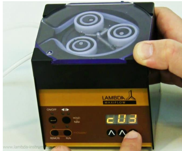
Figure 2-18 If you wish to repeat the same program 3 times, increase the cycle number to " c03 " by pressing the buttons ^ ^ ^ below the display (from 0 to 99 cycles). The program can be repeated up to 99 times, indicated by " c99 ". If 0 is entered for the cycle number " c00 ", the program will run continuously (infinite loop).
