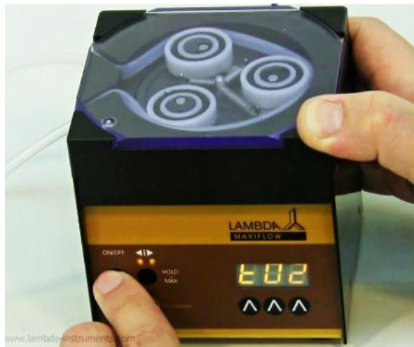
Figure 2-12 Press the ON/OFF button again, the symbol “t02” will briefly appear on the display.
