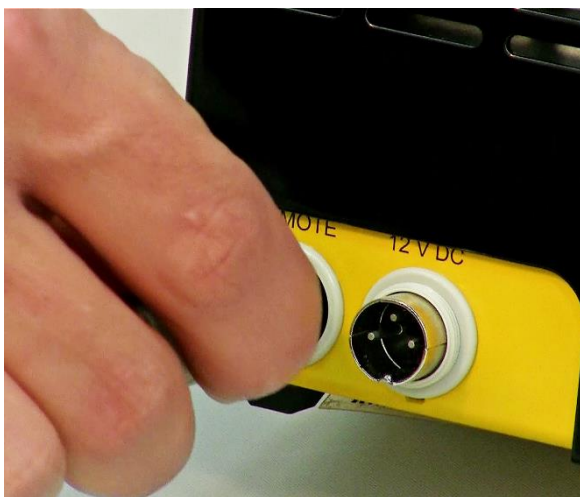
Figure 4-1 For remote control, connect the 8-poles Pump remote control cable into the 'Remote' socket at the rear of the Peristaltic Pump.
