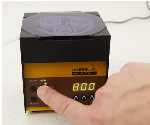
Figure 1-14 LED illumination in the direction |▶ represents the anticlockwise rotation.
