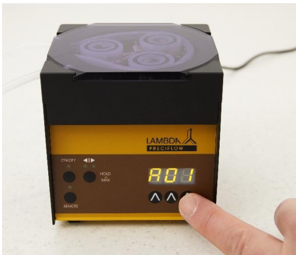
Figure 4-5 To change the address press the buttons ▲ ▲ ▲ under the display until the desired number is obtained.
