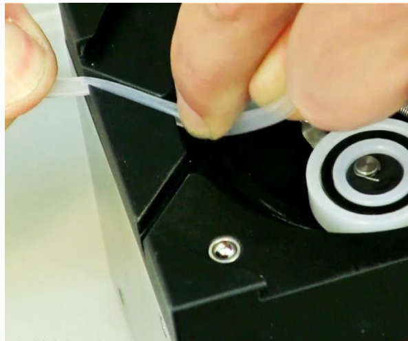
Figure 1-6 Press the tubing into the back slot on the top of the peristaltic pump. Thin tubing should be pushed completely to the bottom.
