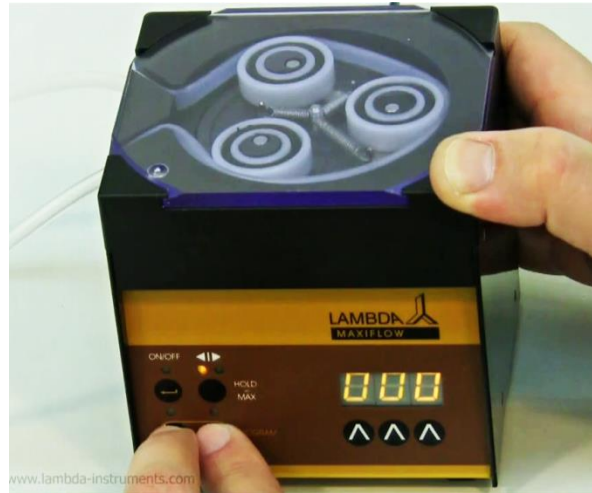
Figure 2-16 The flow rate (000) of the next step which will not be programmed appears on the display.
