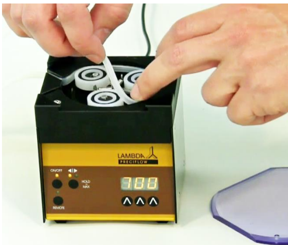
Figure 1-7 Guide the tubing around the slowly turning plastic bearings towards the front slot.
