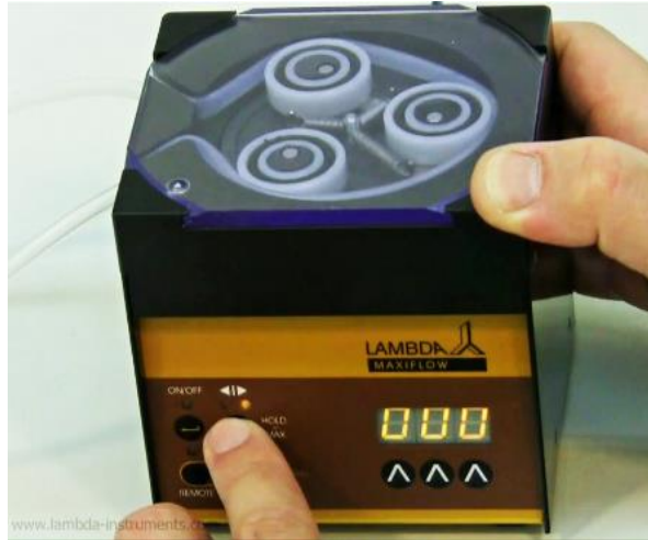
Figure 2-10 Select the direction of the pump rotation using the direction button ◀▶ for each flow rate program.
