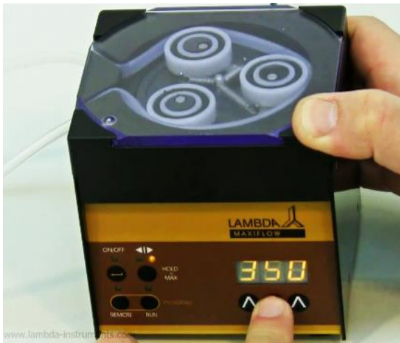
Figure 2-5 Set the desired flow rate value for the first program step by pressing the buttons ▲▲▲ below the display (from 0 to 999, corresponding to 0 to 100% of the motor rotation speed).
