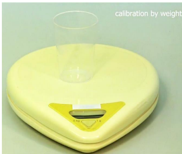
Figure 3-3 Measure the weight of the empty beaker using a sensitive weighing scale. For the exact measurement of the liquid collected, tare the weighing scale with the measuring beaker (Example: 0.000 g).
