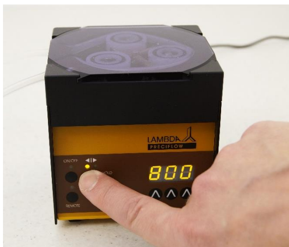
Figure 1-13 LED illumination in the direction ◀| represents the clockwise rotation.
