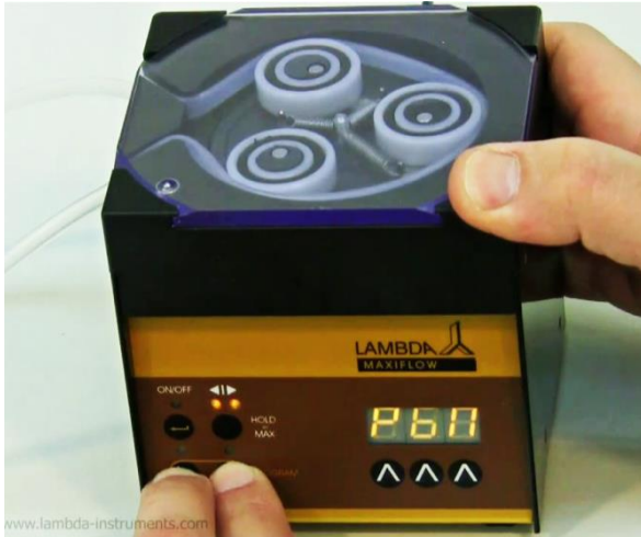
Figure 2-1 Press the REMOTE and RUN simultaneously until the indication “ PGM ” appears on the display.
