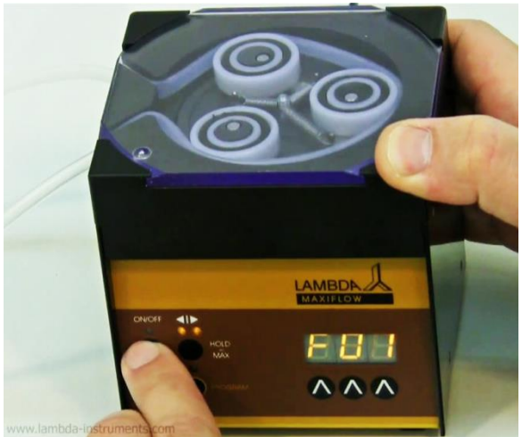
Figure 2-3 Press the ON/OFF button. The indication “ F01 ” will appear for a short time on the display indicating that you can select the first flow rate (speed setting) value.
