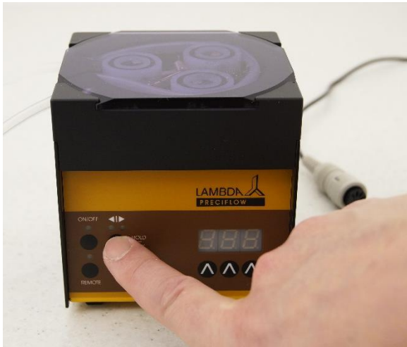
Figure 4-3 Disconnect the pump from the mains. While keeping the direction button ◀▶ pressed connect the pump to the mains again.
