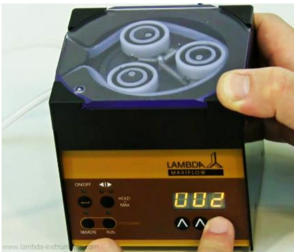
Figure 2-13 Set the time of the second program step.
