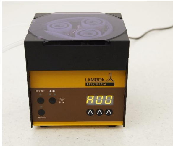
Figure 3-4 The message “A” and two numbers will appear on the display. This number from 00 to 99 is the current address of the pump.
