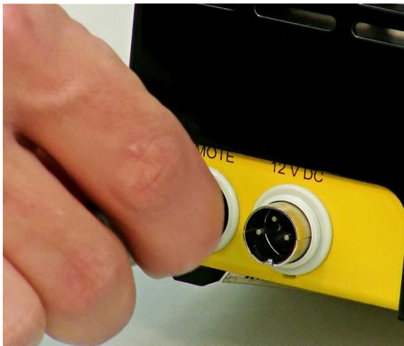
Figure 3-1 For remote control, connect the 8-poles Pump remote control cable into the 'Remote' socket at the rear of the Peristaltic Pump.
