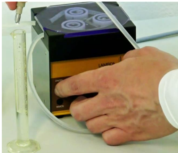
Figure 2-3 Exactly after 60 seconds, switch off the pump.
