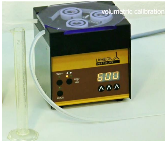
Figure 2-1 Connect the tubing to the liquid from a source and set the desired speed (e.g. 600). Keep the measuring cylinder ready.
