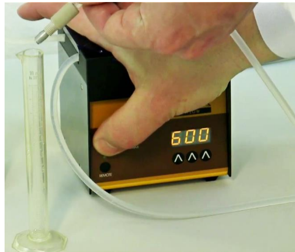
Figure 2-2 Turn on the pump and have the other end of the tubing ready near the measuring cylinder. Carefully collect the liquid being pumped in the measuring cylinder for about 60 seconds.
