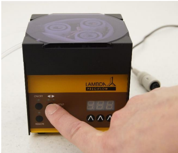
Figure 3-3 Disconnect the pump from the mains. While keeping the direction button ◀▶ pressed connect the pump to the mains again.
