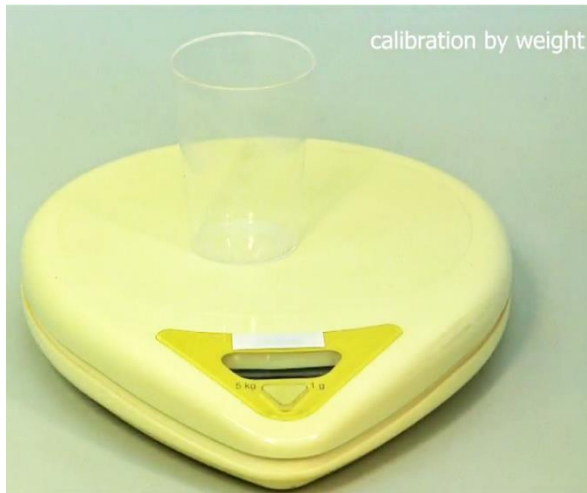
Figure 2-5 Measure the weight of the empty beaker using a sensitive weighing scale. For the exact measurement of the liquid collected, tare the weighing scale with the measuring beaker (Example: 0.000 g).
