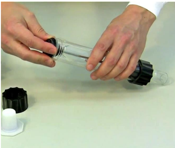
Figure 1-7: Place the centering part with the rubber seal on the axis of the distributor.
