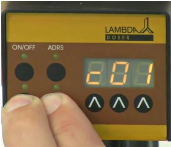
Figure 2-13: Press both REMOTE and RUN buttons simultaneously and you will see the indication “c01” on the display. This indicates that the program will be executed only once and the powder dosing instrument will stop afterwards.
