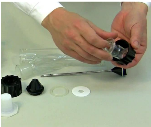
Figure 1-1: The ground glass piece is put through the threaded screw cap SVL 42.
