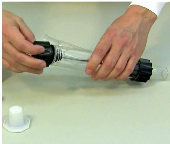
Figure 1-8: Secure the centering part with through the axis of the distributor with the screw cap to the glass vessel.
