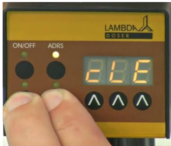
Figure 2-2: Continuous pressing of Remote and Run button even after the indication of “ PGM ” ends up with the “ cLE ” indication.
