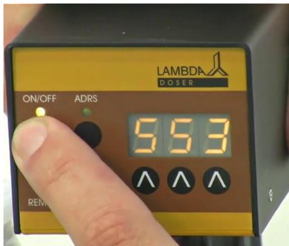
Figure 1-14: Pressing On/Off button on the motor unit after choosing the dosing speed.
