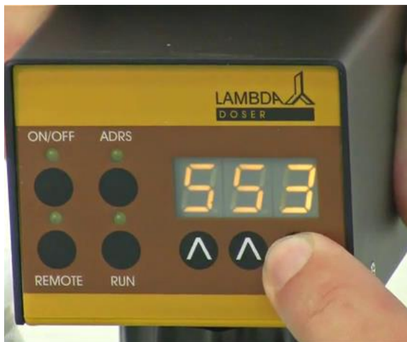
Figure 1-13: Choosing the speed of powder addition with the help of control buttons \wedge \wedge \wedge .
