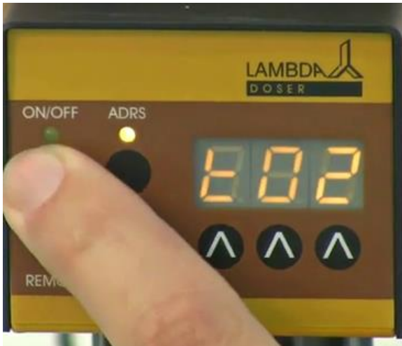
Figure 2-9: Press the ON/OFF button again. The symbol “t02” will briefly appear on the display.
