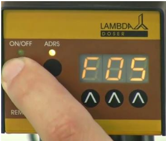
Figure 2-11: After having entered the time of the last step, press the ON/OFF button. The flow rate (000) of the next step which will not be programmed appears on the display. For example: “F05”
