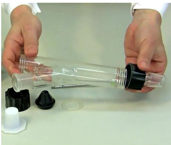
Figure 1-3: The screw cap with the Teflon disc and ground glass piece is screwed to the Doser glass vessel with one side arm.
