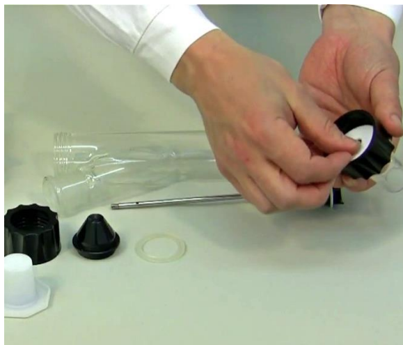
Figure 1-2: The Teflon disc is put inside the screw cap and placed on the ground surface of piece.
