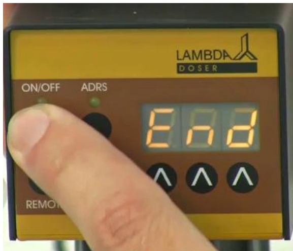
Figure 2-15: Press the ON/OFF button again until the indication “ End ” appears on the display to confirm and save the program.
