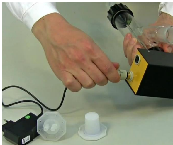
Figure 1-11: The 12 V connector of the power supply is plugged into the 12 V DC socket of the motor unit and the power supply is connected to the mains.
