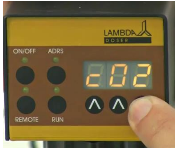
Figure 2-14: If you wish to repeat the same program 2 times, increase the cycle number to “c02” by pressing the buttons ^ ^ ^ below the display (from 0 to 99 cycles). The program can be repeated up to 99 times, indicated by “c99” . If 0 is entered for the cycle number “c00” , the program will run continuously ( infinite loop ).
