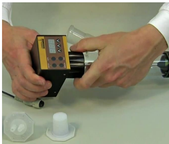
Figure 1-10: Press the axis of the motor unit completely inside the centering part. So that the metal pin of the motor unit will fit into one of the
