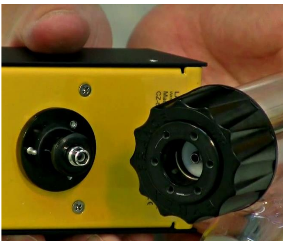
Figure 1-9: Axis of the motor unit with metal pins and the centering part with six holes.
