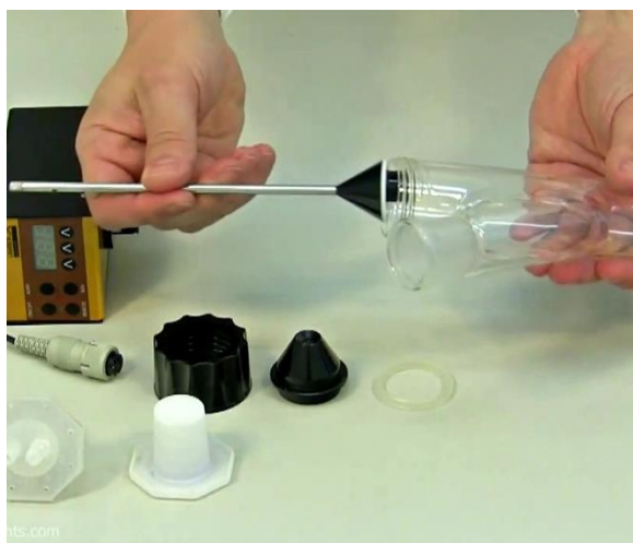
Figure 1-4: The distributor (standard) is inserted inside the glass tube with its opening directed downwards so that it will not be damaged.
