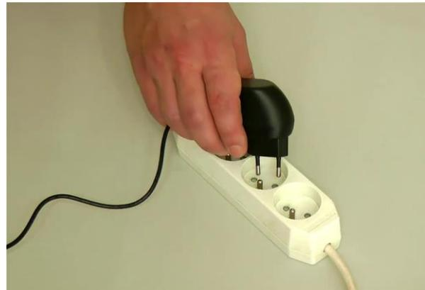
**Figure 1-2** Plug the universal switching power supply into the mains (90–250V/50–60 Hz). After a short beep signal the display will be illuminated. The last used settings will appear on the display.
