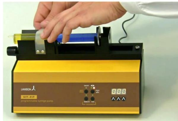
**Figure 1-8** Secure the body of the syringe using the elastic fixation band.
