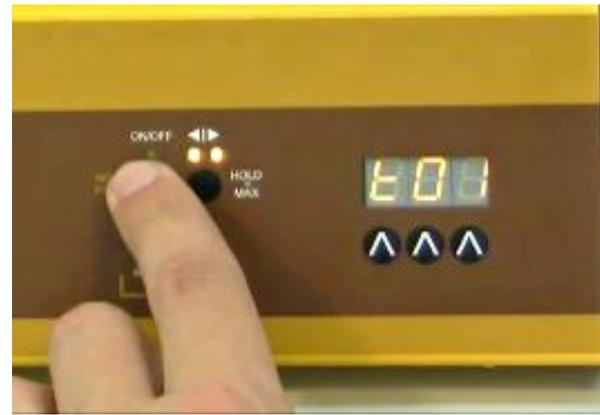
**Figure 2-6:** Press the **ON/OFF** button. The indication “t01” will appear for a few seconds on the display indicating that you can program the time period of the first step.
