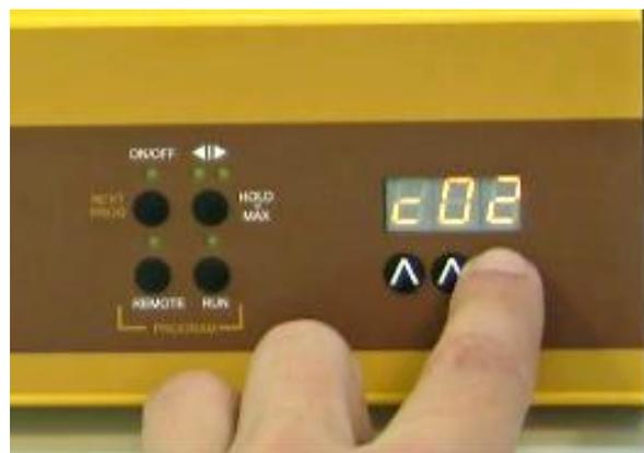
**Figure 2-16:** If you wish to repeat the same program 2 times, increase the cycle number to “**c02**” by pressing the buttons **^ ^ ^** below the display (from 0 to 99 cycles). The program can be repeated up to 99 times, indicated by “**c99**”. If 0 is entered for the cycle number “**c00**”, the program will run continuously (**infinite loop**).
