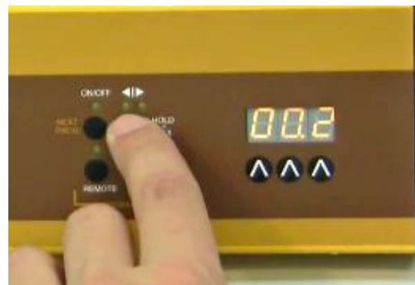
**Figure 2-8:** By pressing the (◀|▶) **direction button**, the time resolution can be set in minutes or 0.1 minutes. In the 0.1 minute time resolution a dot is displayed, e.g. “00.1”. The time resolution can be set individually for each program step.
