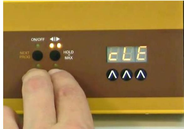
**Figure 2-2:** Continuous pressing of Remote and Run button even after the indication of "PGM" ends up with the "cLE" indication.
