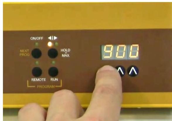
**Figure 2-4:** Set the desired flow rate value for the first program step by pressing the buttons ▲▲▲ below the display (from 0 to 999, corresponding to 0 to 100% of the motor rotation speed).
