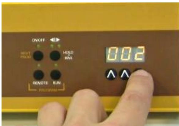
**Figure 2-7:** Select the desired time period for the first program step by pressing the buttons ▲▲▲ below the display (from 000 to 999 minutes or 00.0 to 99.9 minutes).
