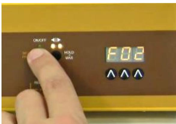
**Figure 2-9:** Press the **ON/OFF** button. The indication “F02” will briefly appear on the display.
