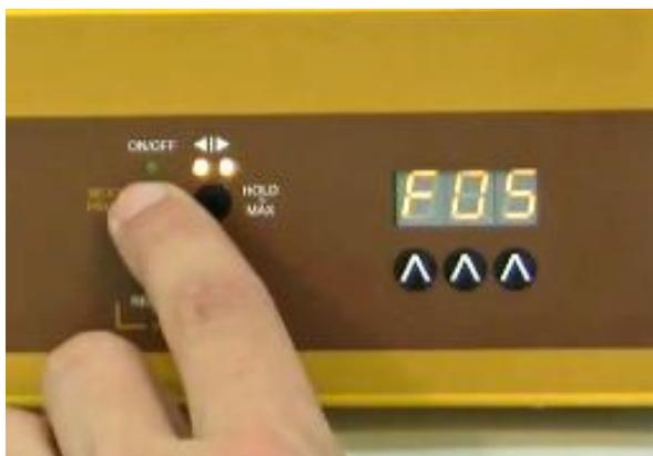
**Figure 2-13:** After having entered the time of the last step, press the **ON/OFF** button. The flow rate (000) of the next step which will not be programmed appears on the display. For example: “F05”
