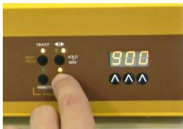
**Figure 2-18:** To **START** the program, press the **RUN** button. The **RUN** and **ON/OFF** LEDs are on.
