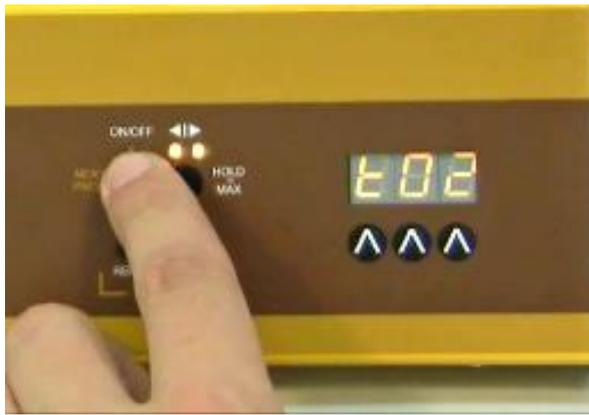
**Figure 2-11:** Press the ON/OFF button again. The symbol “t02” will briefly appear on the display.
