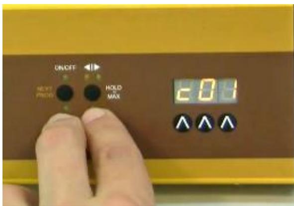
**Figure 2-15:** Press both **REMOTE** and **RUN** buttons simultaneously and you will see the indication “**c01**” on the display. This indicates that the program will be executed only once and the syringe pump will stop afterwards.
