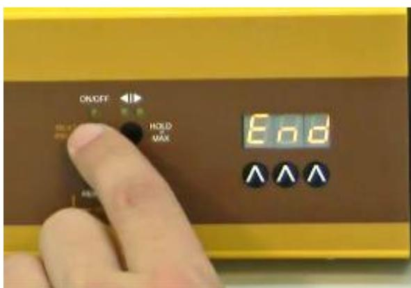
**Figure 2-17:** Press the **ON/OFF** button again until the indication “**End**” appears on the display to confirm and save the program.
