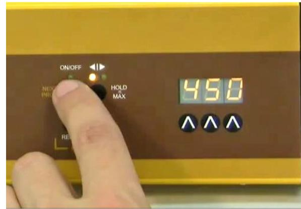
**Figure 1-10:** Pressing On/Off button after choosing the speed.
