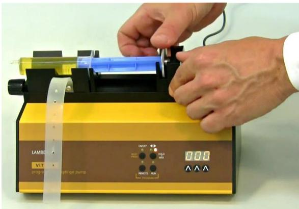
**Figure 1-7** Rotate the fixing disc (clockwise) to restrict the movement of the plunger extremity.
