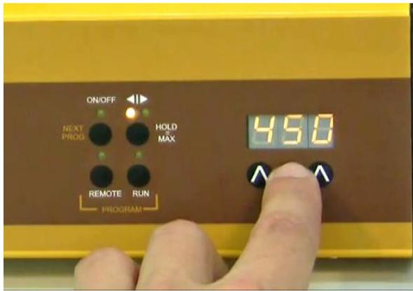
**Figure 1-9:** Choosing the speed of motor with the help of control buttons  $\blacktriangle\blacktriangle\blacktriangle$ .
