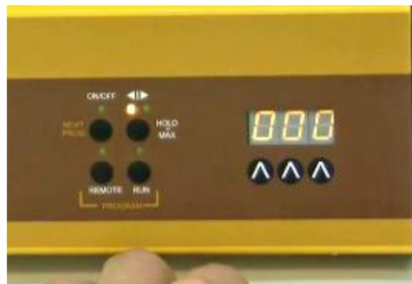
**Figure 2-14:** Do not change the flow rate (000).
