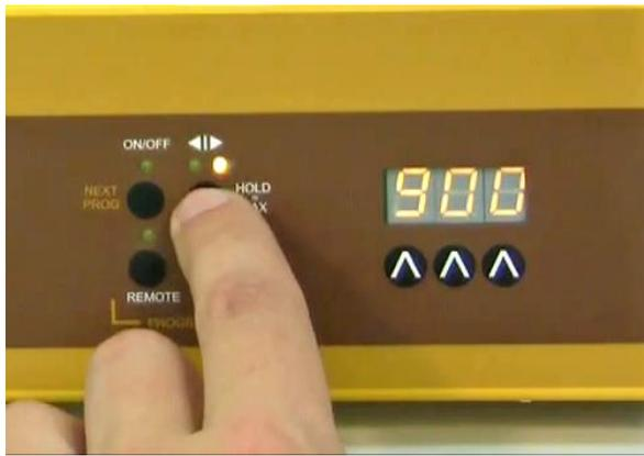
**Figure 2-5:** Select the direction of pusher movement (delivery or filling) using the direction button (◀|▶).
