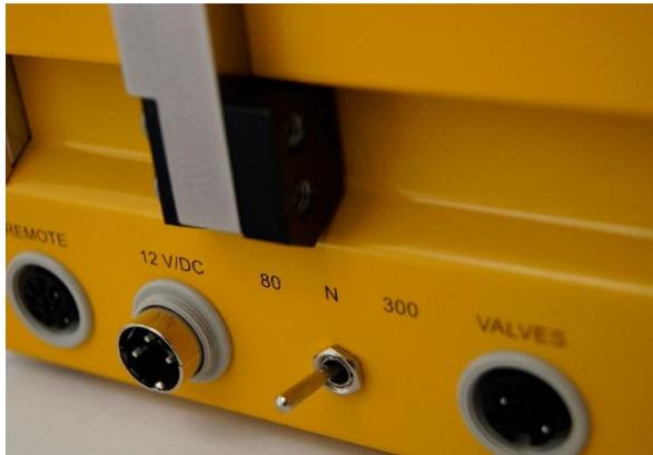
**Figure 1-1** Plug the power supply connector into the corresponding socket (12 V/DC) at the rear of the syringe pump and secure it in place by rotation of the ring.
