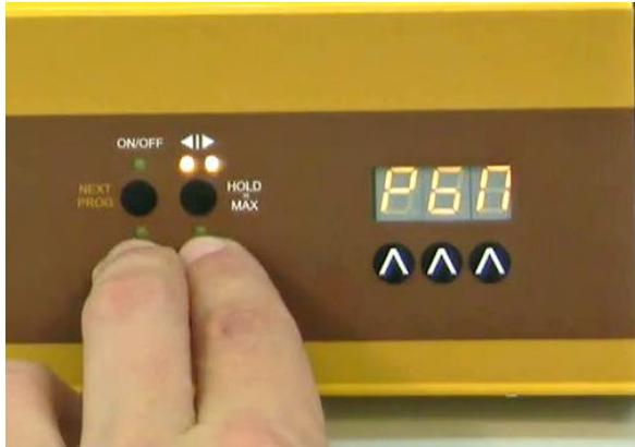
**Figure 2-1:** Pressing Remote and Run buttons simultaneously and the "PGM" indication appears.
